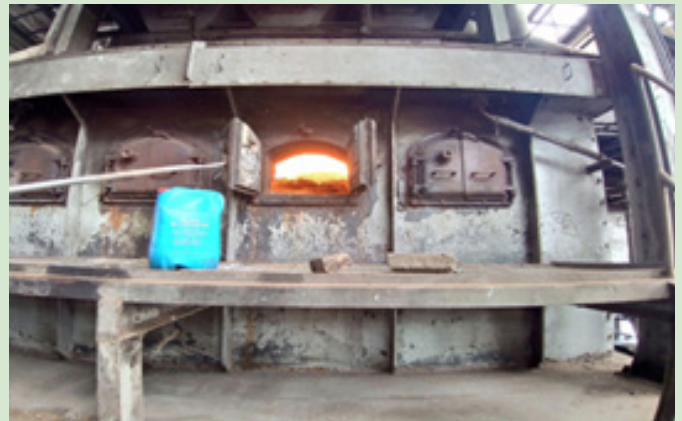
Biomass combustion furnace at GOPDC
