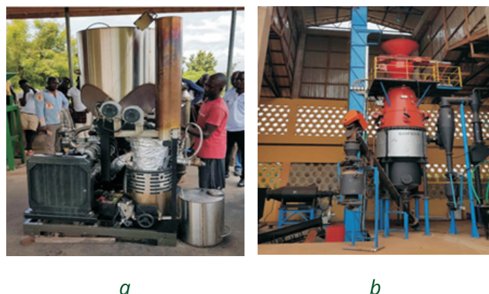
Figure 40: a) 20 kW gasifier plant at Papasi and b) 120 kW gasifier plant at Asueyi
