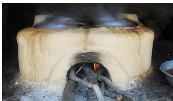
Figure 45: The use of Firewood in improved cookstoves for Beer Brewing in Burkina Faso
